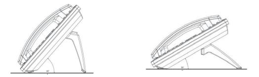
To attach the stand to the phone you will see 2 sets of slots on the rear of the telephone base and 2 sets of notches on the top of the stand (marked A & B in the diagram beow). For illustration purposes we are using the 50 degree angle set up.
