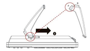
A to A gives a 50 degree tilt B to A gives a 30 degree tilt
